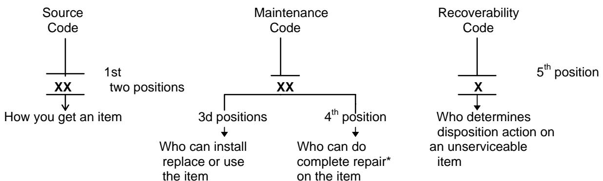
\*Complete Repair: Maintenance capacity, capability, and authority to perform all the corrective maintenance tasks of the "Repair" function in a use/user environment in order to restore serviceability to a failed item.
